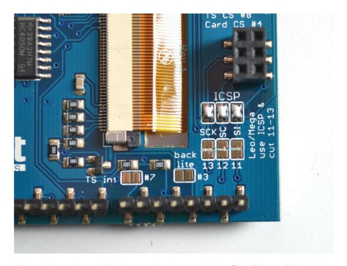
You can then cut the small line in between the #11, #12, #13 pads. This will free up digital #11, 12, and 13 for you to use on the Leo or Mega.
