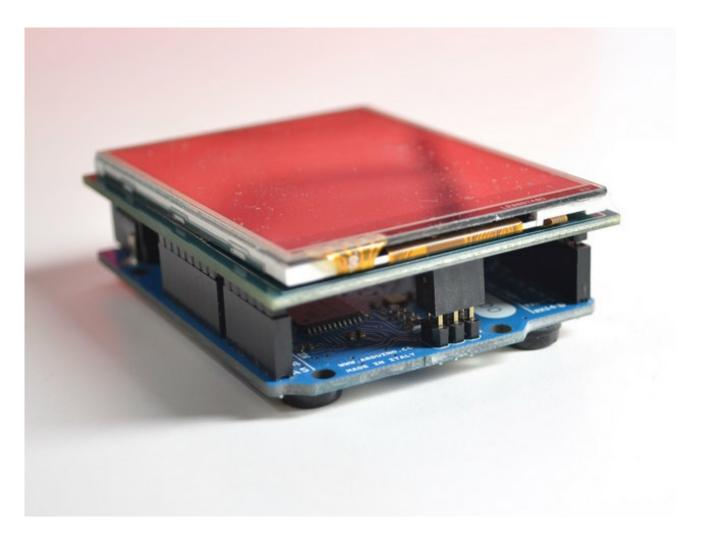
With this mod, the shield uses the ICSP header for data so make sure your duino (or stack of shields) has a ICSP plugged into the socket as above!
