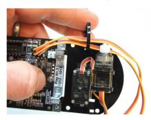
17. Use the slots on the other side of the body to thread another cable tie and secure the wires on the other side as shown. The wires are longer than they need to be, so it requires some artistic arranging. Do not tighten this cable tie fully either.
