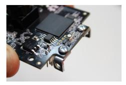
13. Take two nylon bushings and press them into the non-threaded holes in these brackets.
