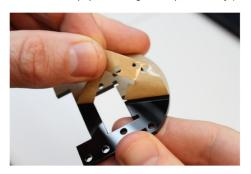
5. Fit one of the servo mounting tab into the slot on the pan/tilt body.
