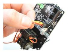
16. Use a cable tie to secure the wires to the body as shown. String the cable tie through the single slot in the body and around the outside. Do not tighten the cable tie fully yet.
