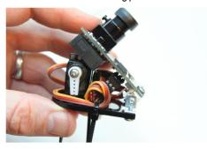
19. When you're happy with the cable situation, make the ties snug, but not too tight (to save the wires) then flip over the assembly and clip the ends of the cable ties.
