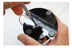
25. Place a short 4-40 fastener through the eyelet of the wire pushrod and attach it to a two-threaded bracket, but don't tighten fully. The pushrod needs to be able to pivot around the screw. Attach the pushrod and fastener to the
