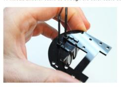
8. Tighten both cable ties by using pliers. It requires quite a bit of force to fully tighten!
