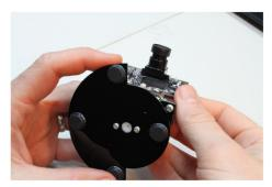
24. Find one of the **servo** horn fasteners in one of the servo baggies and attach the base to the body. (Here, the wide part of the base is facing forward, which should be close to the center of travel.)
