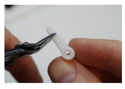
2. Put the servo horn on the servo and check both ends of travel. You can do this by moving the horn all the way to the right:
