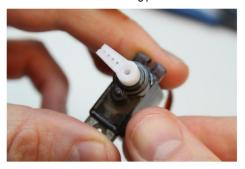
and adjusting the mounting angle of the horn such that the center of travel has the servo horn pointing downwards. Note, it's OK to move the servo in this way even though it requires a fair amount of force. And it makes a cool sound!
