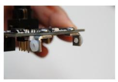
14. Slide the Pixy into the body assembly. Use two **long 4-40** fasteners and insert them from the outside as shown in the picture. The 4-40 fasteners will form an axle for Pixy to use for tilting. Make sure that the brackets are mounted squarely--- this can cause binding. Tilt Pixy back and forth a couple times and make some adjustments if you feel some binding.
