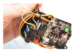
18. Verify that there is enough slack in the cables to allow Pixy to tilt fully forward and backward.
