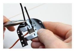
9. Take the 2nd servo and place in the other hole in the body as shown in the picture. Note that the wires for the servos are pointing in opposite directions.
