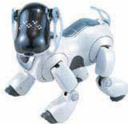
Figure 13. The low-cost four legged robot AIBO
