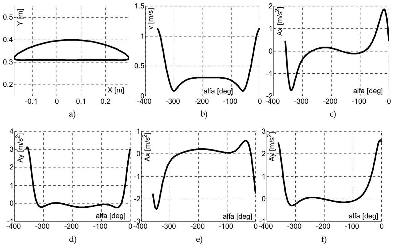
Figure 24. Simulation for the walking characteristics of the 1-DOF leg in Fig.23 with  $p=20$  mm and  $h=30$  mm: a) Point C trajectory; b) Point A velocity; c) Acceleration  $a_{Ax}$ ; d) Acceleration  $a_{Ay}$ ; e) Acceleration  $a_{Ax}$ ; f) Acceleration  $a_{Ay}$
