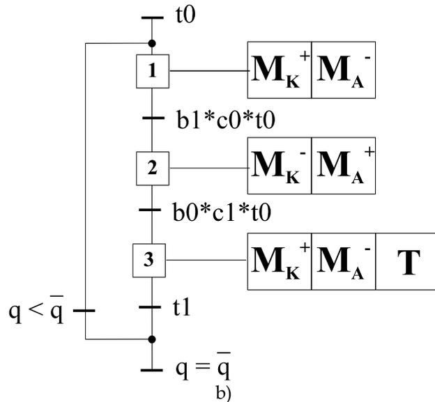
Figure 27. An example of the operation programming for the proposed low-cost anthropomorphic wheeled leg in Fig.26 for the straight walking: a) flowchart of elementary actions; b) Grafcet for PLC programming
