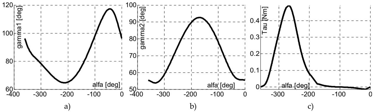
Figure 25. Simulation for the walking characteristics of the 1-DOF leg in Fig.23 with  $p=20$  mm and  $h=30$  mm: a) Transmission angle  $\gamma_1$ ; b) Transmission angle  $\gamma_2$ ; c) actuating torque  $\tau$
