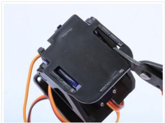
the back of the camera module. Two cuts, as shown in the photos will remove the top left side of the bracket.
